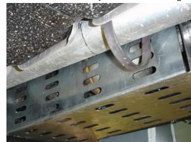
Catalytic Converter Cage to deter the growing problem of catalytic converter theft
