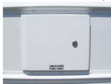
Locking Fuel Door to deter gasoline theft
